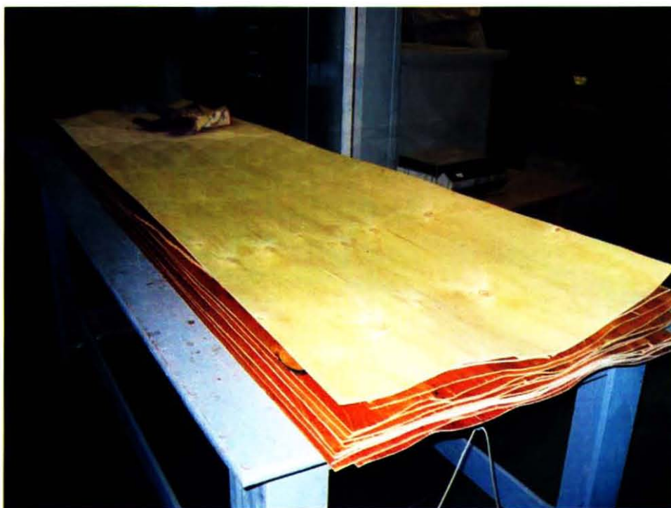
Laid up Pine panel ready for hot pressing.
