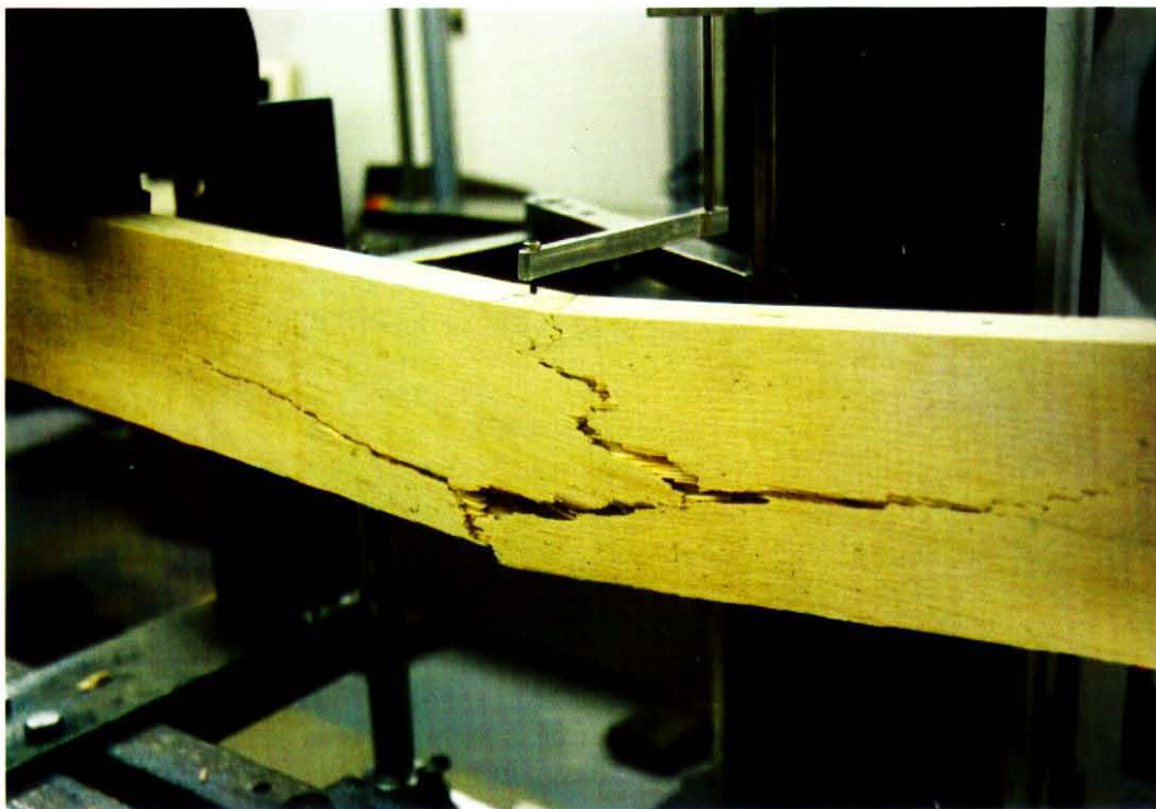
Typical Radiata Pine failure in edgewise bending.
