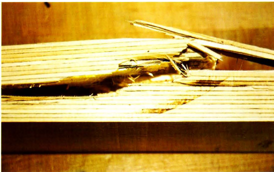
Typical Radiata Pine failure in flatwise bending.
